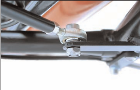
Scorpion / Scorpion fx: The rod end is mounted on top of the handlebar sheetmetal bracket with a washer in between.
