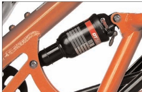
Air Shock DT-Swiss XM180 Damping ist adjusted with the red knob at the rear end. The shock must be installed with the lock-out lever on the backside facing down to avoid a collision between lever and frame when the suspension is moving.
