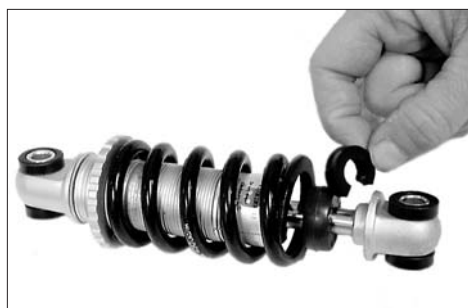
The suspension travel is adjusted by adding clips to the piston rod of the spring element.
