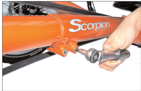
Unscrew the clamping bolts to adjust the front boom.
