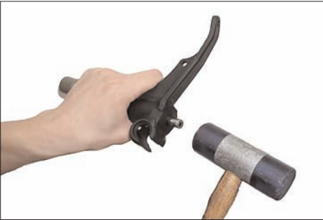
A hammer blow on the auxiliary bolt releases the piston inside the knuckle.
