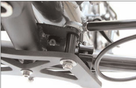
Scorpion fs: A washer must be located between rod end and the sheetmetal bracket.
