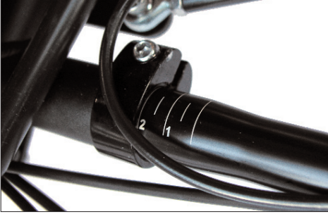
Handlebar width and angle are adjusted with the clamp at the stem under the main frame.
